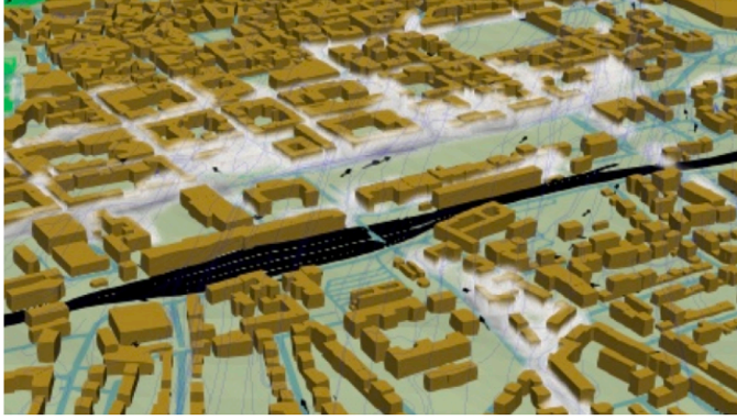
Fig. 3. Visualization of pollution dispersion in the Urban Air Project use case modeling the city of Győr. Streamlines and vectors indicate air flow direction, while white cloud shows pollution spread.
