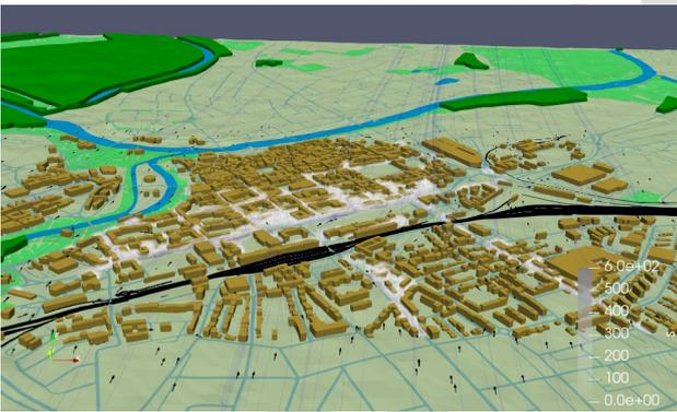
Figure 2: Visualisation of simulation results of the UAP-FOAM model within the city of Győr. Geometric representation of buildings (brown), ground (grey), etc. come from the original city geometry, not the simulation mesh. Air flow is depicted with streamlines, while vectors indicate flow direction. Pollution concentration is indicated by the grey fog between the buildings. Lighter and darker colours indicate lower and higher concentration of pollution.
